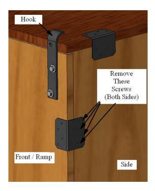
Remove the Front/Ramp, swing it down, and...
